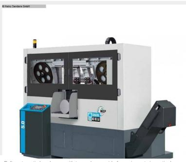
Fully automatic band saws with two-column guide for series cuts in particular materials that are difficult to machine and solid material.
