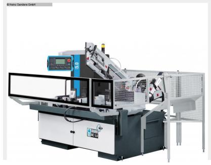
Powerful miter band saw for cuts from 45 ° right to 60 ° left
