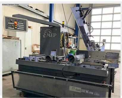
Powerful miter band saw for cuts from 45  $^{\circ}$  right to 60  $^{\circ}$  Left
