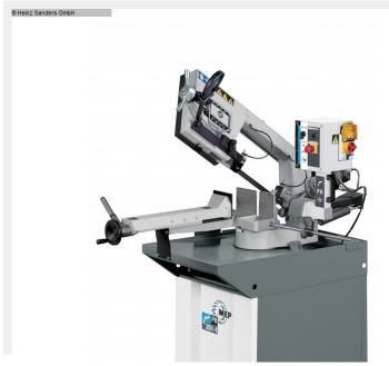
Compact, powerful workshop miter band saw machine for cuts from 0  $^{\circ}$  to 60  $^{\circ}$  left
